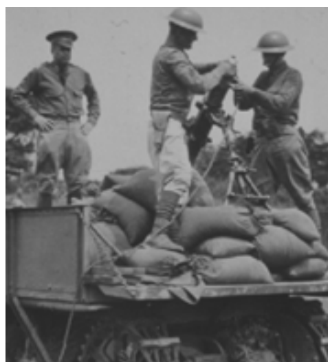
Fig. 2-24. A 4.2-in. chemical mortar mounted on a light cargo carrier in 1928. The carrier had a speed of 20 mph. Photograph: Chemical and Biological Defense Command Historical Research and Response Team, Aberdeen Proving Ground, Md.
